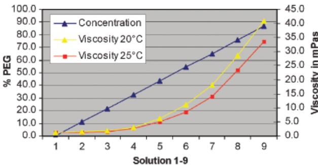
FIG. 1—Polyethylene glycol (PEG) concentrations and graphical delineation of the resulting viscosities (at 20°C and at 25°C). At higher temperatures, the content of PEG needs to be increased to reach the same viscosity.
